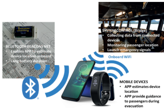
Figure 13. Schematic view of the pilot arrangement and communication between components
